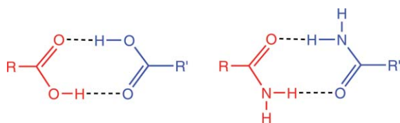
Fig. 3 The -\text{COOH}\cdots\text{HOOC}- or -\text{CONH}_2\cdots\text{H}_2\text{NOC}- binding motifs impart no additional degrees of freedom to the attached groups R and R' because rotation of the binding motif around the \text{R}\cdots\text{R}' axis has no effect on the relative position of R and R'.
